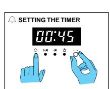
Press button B and while turning knob A enter the required time (max. 23 h 59 min.). After required time has been selected the clock will revert to the time of day. When time is up an audible signal will be heard for approx 2 mins. To cancel press button B and return control and thermostat knobs to 'O' OFF.
